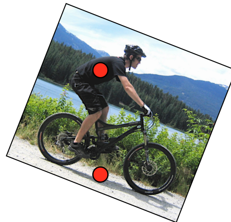
Picture 2.2e: To counter-act this, the rider now moves his hips over the rear of the bike into the BACK POSITION. In this position, the rider is rear-heavy on the flat ground, but nice and centered when pointing downhill, whilst the BRAKES ARE APPLIED. Even though the rider has moved over the rear wheel, both wheels are evenly weighted (right picture).
