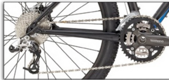
PICTURE 1.1A: GEAR RATIOS - THE CHAIN ON THIS BIKE IS PLACED ON THE HARDEST GEARS FRONT AND BACK.
