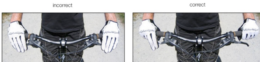
PICTURE 1.1C: BRAKING FINGER POSITION (RIGHT BRAKE IS THE REAR FOR THIS BIKE)
